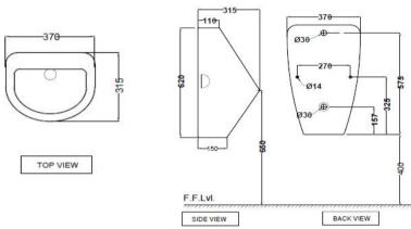
ALL DIMENSIONS ARE IN MM. (TOLERANCE ± 5 MM)
